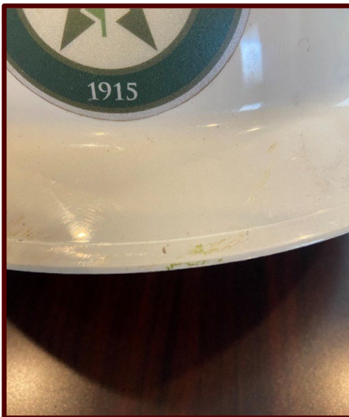
Smudge where limb impacted FAL3 Trainee's hard hat and knocked it off his head
